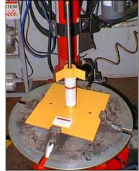
#38600 shown secured to rim clamp machine.
