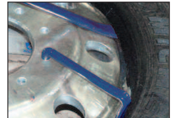
• Curved end For mounting and demounting top bead
