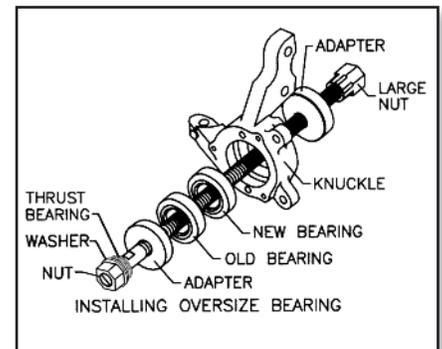
6. Installing Oversized Bearing
