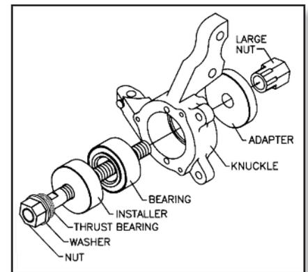
3. Installing Bearing
