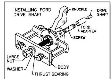
7. Installing Ford Drive Shaft
