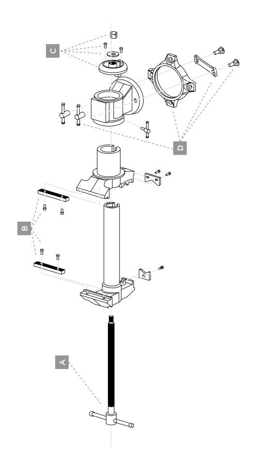
KEN-TOOL PRO MULTIPURPOSE 5 IN BENCH VISE MAIN SCREW SET JAW PLATE SET END CAP SET SWIVEL BASE SET
