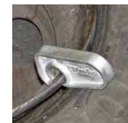
Newest Bead Holder - Made From Aluminum
