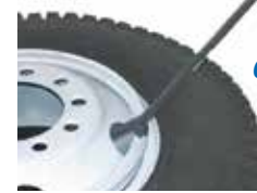
Use for multi-piece wheels, especially hub type.
